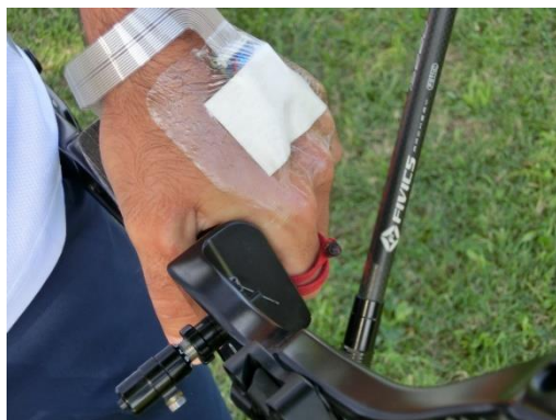
Figure 3: SETUP A - Experimental setup with IMU positioned on the back of the hand.
